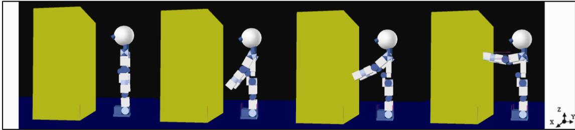
Fig. 15. Sequence of motions for HOAP-3 touching a wall.
